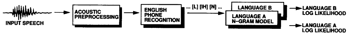
Fig. 2. PRLM block diagram. A single-language phone recognition front end is used to tokenize the input speech. The phone sequences output by the front end are analyzed, and a language is hypothesized.
